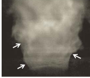
Figure 8 : Line of sight integrated flame luminosity for asymmetric forcing showing presence of helical flame disturbance, reproduced from O'Connor [45].
